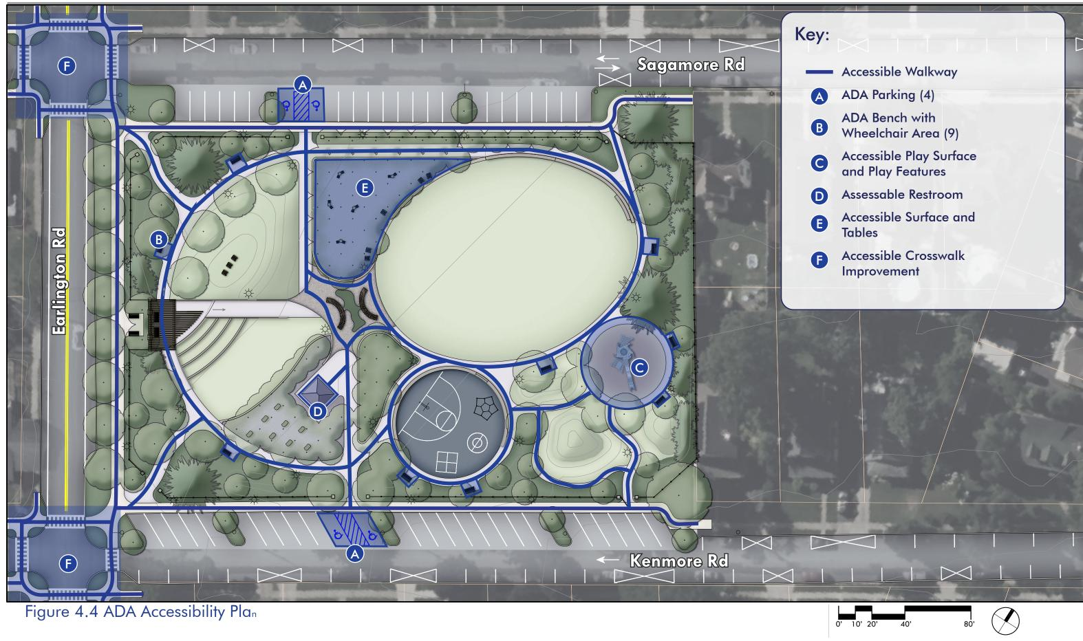
Curb extensions and crosswalks (#6) are proposed at the Earlington Road intersections with Sagamore Road and Kenmore Road. The curb extensions will provide for the existing two 11-foot-wide travel lanes. Crosswalks will be paired with flashing beacons to indicate pedestrian right-of-way to vehicular traffic. As this is a state road, PennDOT will need to be consulted for the design and engineering (and an HOP Permit) for the improvements along Earlington Road.
