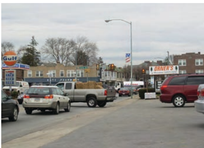
Wide Curb Cuts Should be Narrowed to Provide Increased Safety and Pedestrian Orientation along Eagle Road
